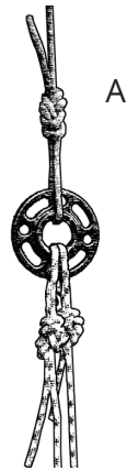
Figure 3. Double stationary: Double ropes attached using retraced figure-8 knots in a stationary rope setup.
