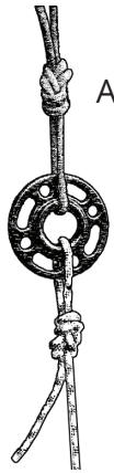
Figure 2. Single stationary: A single rope attached using a retraced figure-8 knot in a stationary rope setup.
